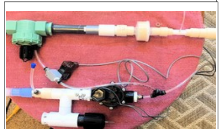
Airway components of the emergency ventilator. [Photo courtesy of Gordon Gibby, KX4Z]
